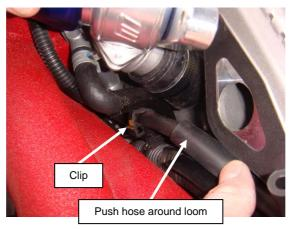
7. Secure the BOV onto the intercooler with the standard bolts and replace the vacuum line to the top of the BOV. (BOV unit may differ)
