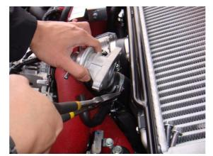
3. Remove the plumb back fitting on the back of the standard BOV and install it onto the Turbosmart BOV using the standard screws. (BOV unit may differ)
