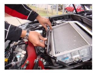
5. Using the provided ½" tee piece, connect the standard oil breather lines on the left hand side of the intercooler in the orientation shown in the picture below and run the provided ½" hose under the intercooler to the oil breather line on the other side of the intercooler, using the provided ½" straight joiner to join the rubber hose to the existing breather line on the right hand side.
